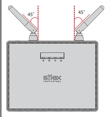
Tilt each antenna outward at a 45 degree angle.
