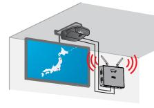
Hang the unit on higher position of the wall to make sure of a good line of sight to terminal devices.
